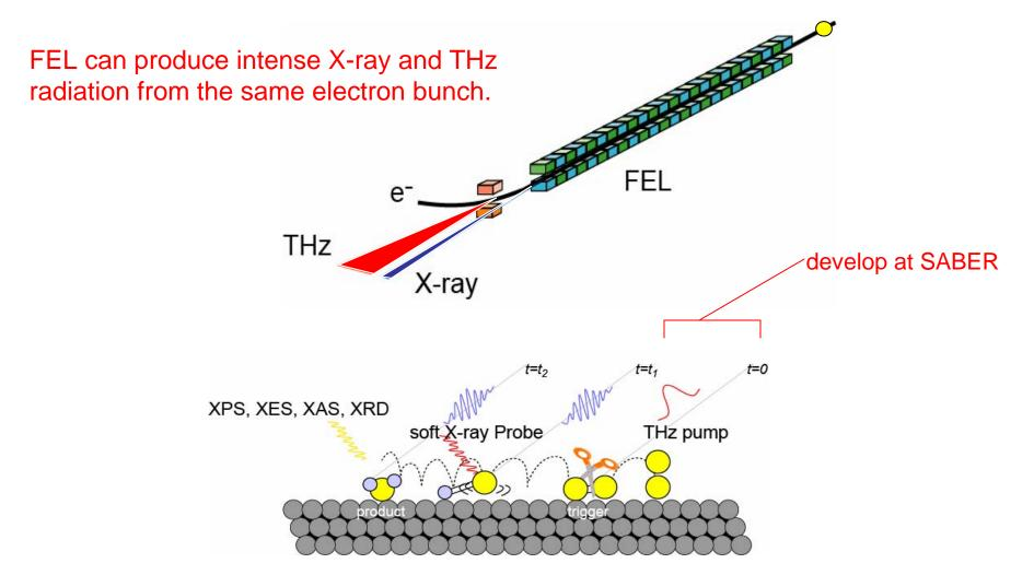
on-axis radiation, soft X-ray, hard X-ray, off-axis radiation: THz **Pump:** THz, **Probe:** XPS, XES, XAS, XRD, IR
