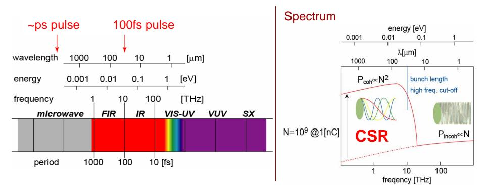
Ultra short electron bunch is necessary for coherent THz radiation. Bunch length = **high frequency** cut-off
