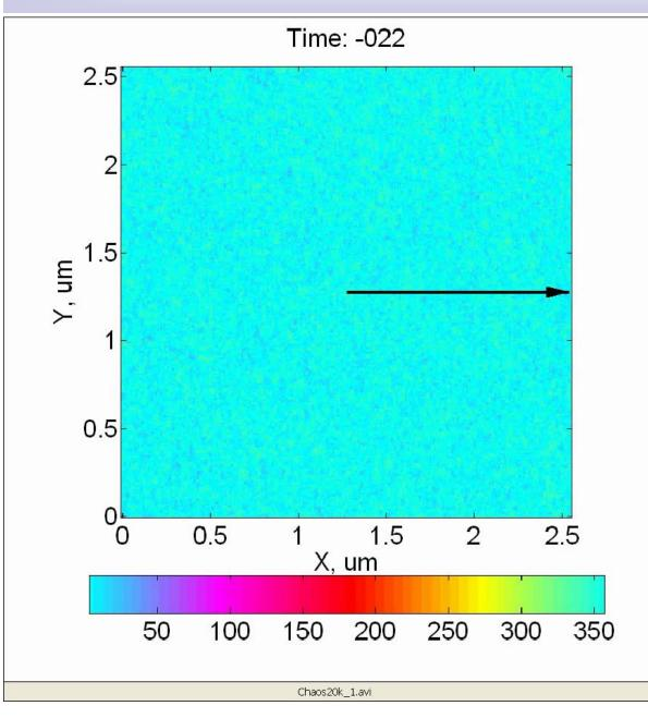
uniform pulse field H<sub>pulse</sub>=20 kOe at ~ 40 um from the center
