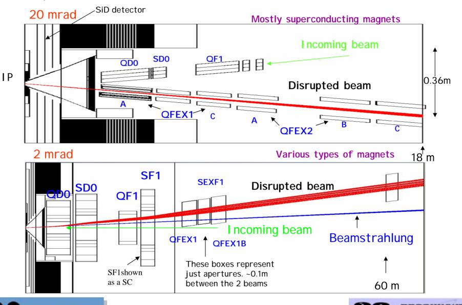
nternational Linear Collider t Stanford Linear Accelerator Center
