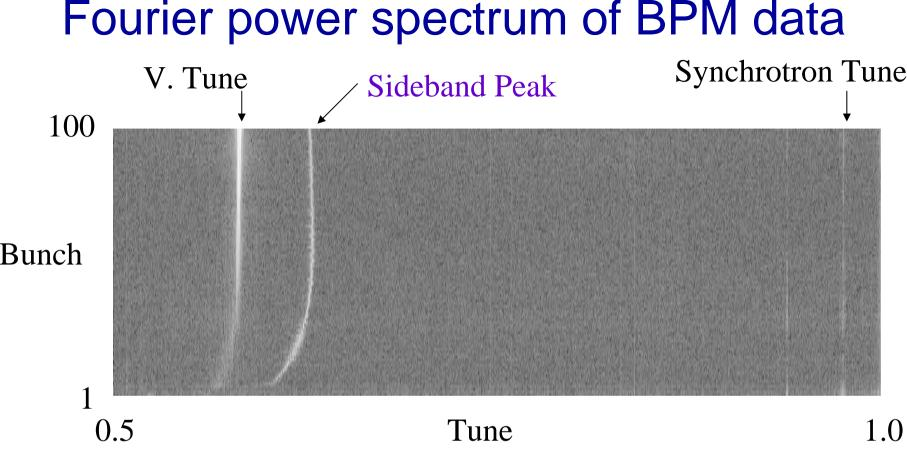
LER single beam, 4 trains, 100 bunches per train, 4 rf bucket spacing Solenoids off: beam size increased from 60  $\mu$ m ->283  $\mu$ m at 400 mA Vertical feedback gain lowered
