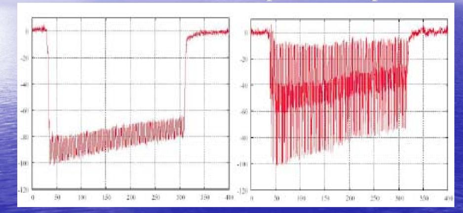
940 μJ/100 pulses with 2.8nsec spacing, UV 266nm, 7psec (FWHM)
