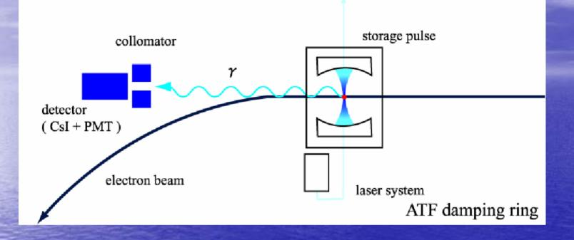
Pulse Laser Wire (Storage laser pulses in optical cavity ):
