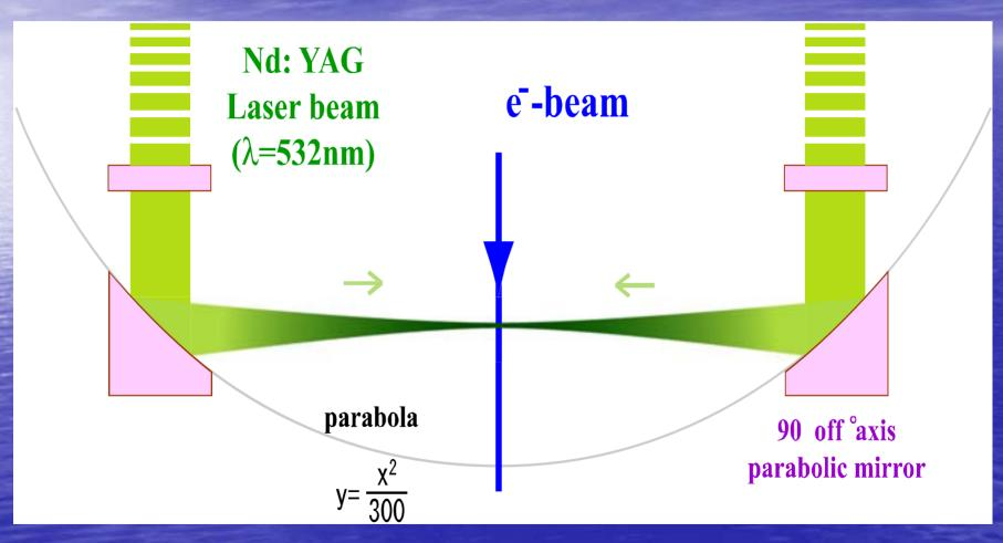
To make  $1\mu$ m(rms) focusing at IP with small crossing angle.
