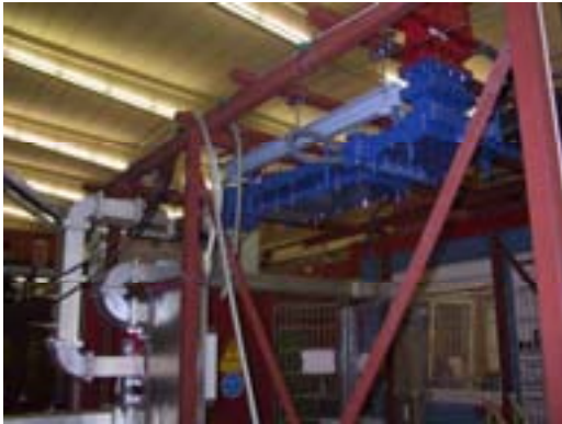
5MW isolator filled with SF 6
