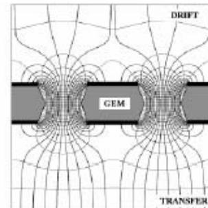
Figure 14 Electric field and equipotential lines in the gas electron multiplier.
