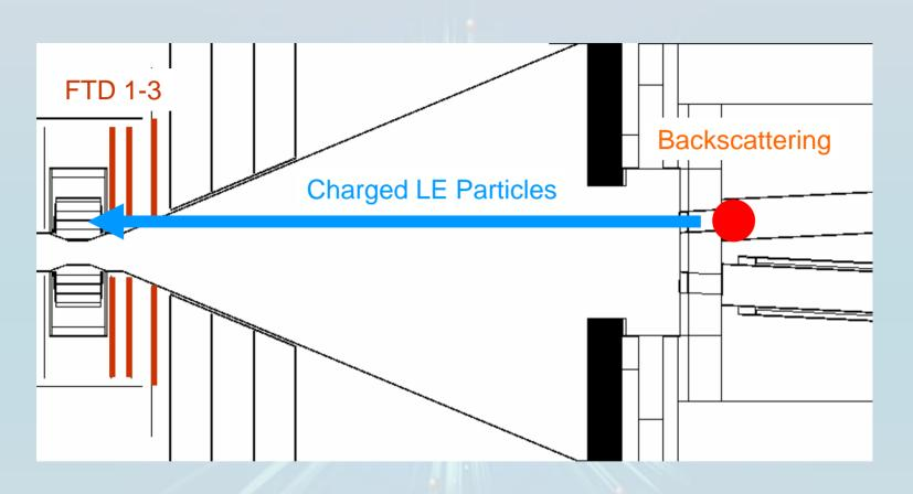
Backscattered particles are collimated by the exit hole and aim directly to the VTX
