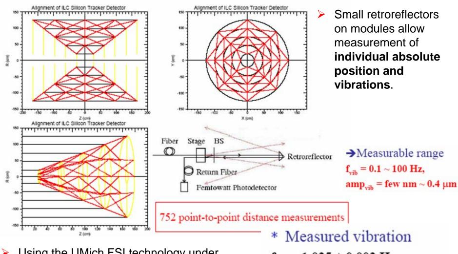
Using the UMich FSI technology under development, the vibrations in a filamentbased structure can be extremely precisely calibrated *in real time*.
