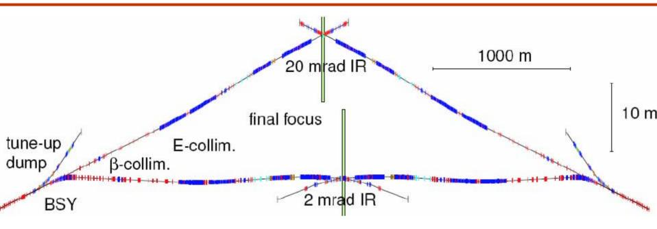
Crossing angle choice correlated with: Detector hall footprint: transverse + longitudinal separation of 2 IR halls Bunch spacing: longitudinal separation of 2 IPs Space for downstream diagnostics
