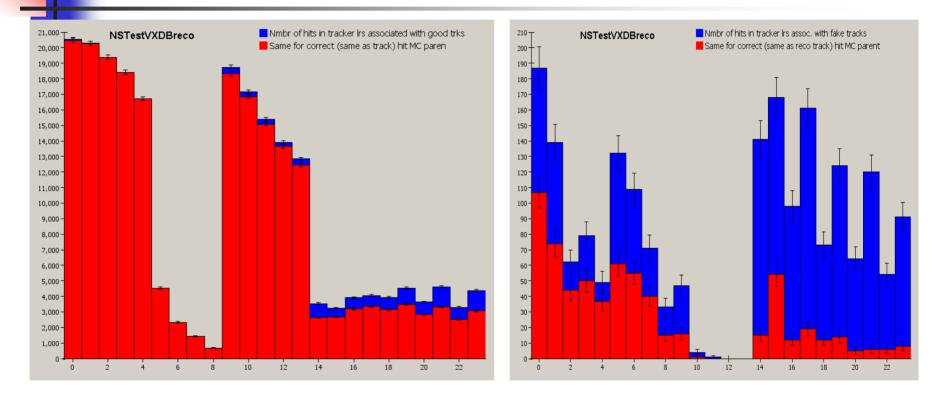
Number of correctly assigned hits for different tracker layers (0-4 barrel VXD, 5-9 – endcap VXD, 10-14 – barrel silicon, 15-24 – endcap silicon layers)
