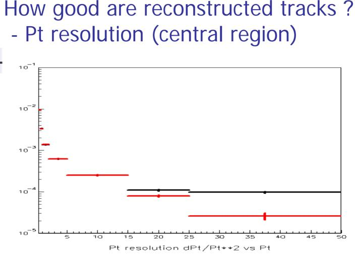
Fitting is not currently implemented for endcap tracks. I need to work on it. So this picture includes only tracks hitting barrel tracker. Black points are for reconstructed tracks without fitting, red – with.
