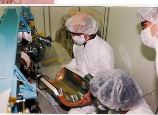
2 halves of barrel F-cage complete the assembly
