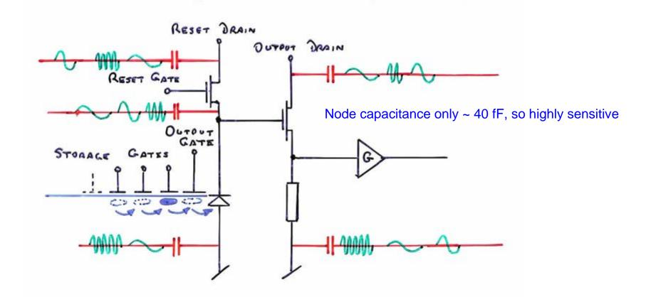
From SLD experience, signal charges stored in buried channel are virtually immune to disturbance by pickup. They were transferred in turn to the output node and sensed as voltages between bunches, when the RF had completely died away
