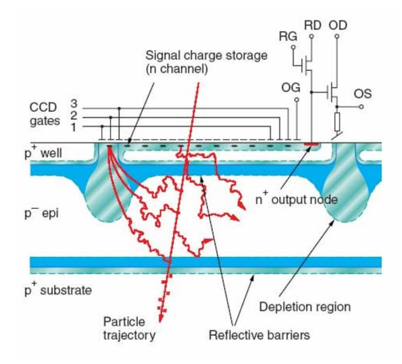
• charge collection to photogate from ~20 mm silicon, as in a conventional CCD
