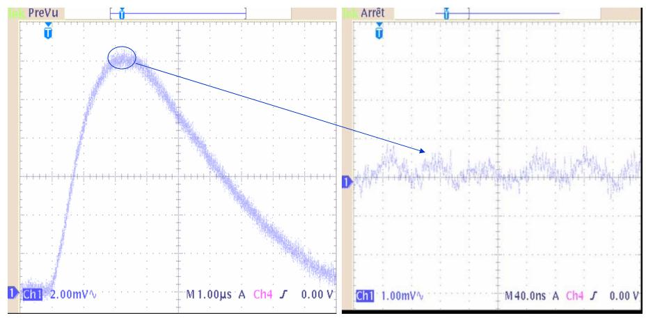
$0.18~\mu m$  readout chip for a silicon tracker 8 MHz oscillations at the shaper output
