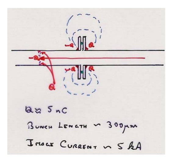
O-ring seals or imperfectly clean metal seals can provide slot antennas through which RF power can pour out, generating precisely the sort of  $\delta$ -function pulse seen by Nick Sinev in SLD
