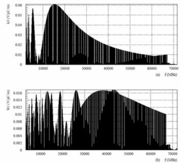
Monopole radiation (above) and dipole (below) Both TE and TM modes are excited for each. Fcy range plotted is 0-70 GHz Peak amplitudes 0.06 and 0.016 V/m per pC respectively Bunch charge is approx 3.2 nC
