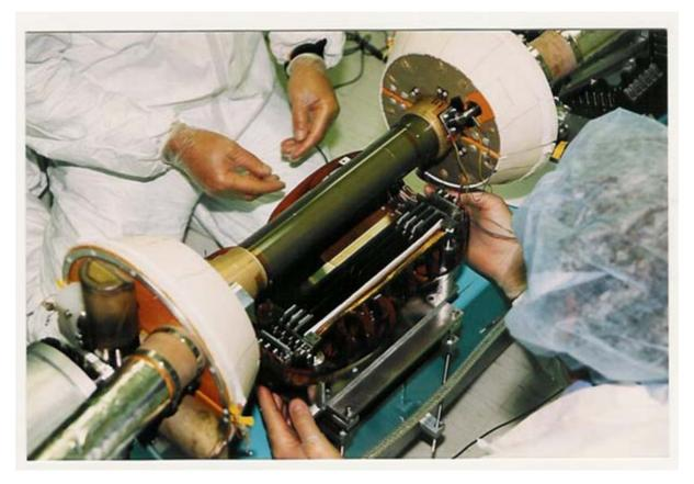
Gas shell, electrically isolated from beampipe, connected by springs to the 4 sections of F-cage endplate ...
