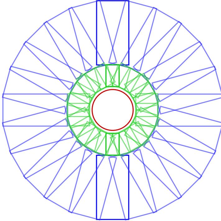
Figure 2: Example layout of the forward disk portion of the vertex detector. The sensors aligned with the vertical axis are a darker shade of green (blue) to illustrate the sensor shape in the inner (outer) annulus
