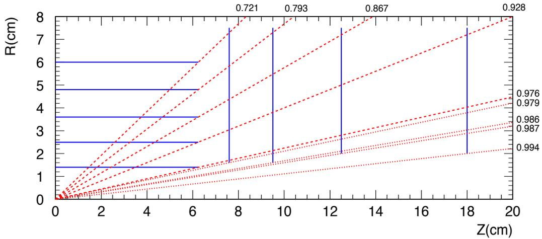
Figure 1: Example layout of the vertex detector. The dashed lines show the acceptance edges of the barrel layers. The dotted lines show the acceptance edges of the forward disks. The black numbers give the value of  $\cos \theta$  associated with each acceptance edge.
