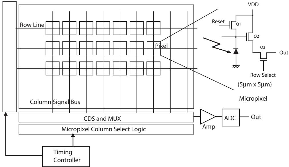
Figure 4: A conceptual diagram showing the layout of the micropixel array and a single micropixel cell.
