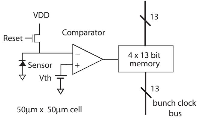
Figure 3: A conceptual diagram showing the layout for one of the single macro pixel cells.
