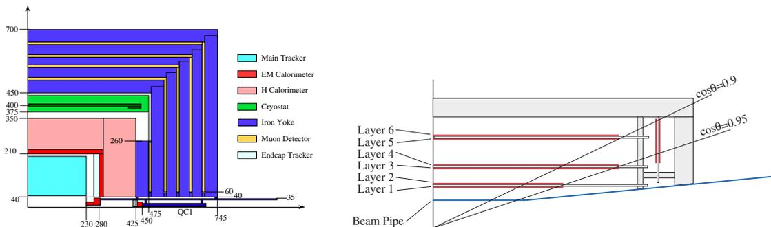
Figure 1: Schematic design of GLD detector model (vertex detector and intermediate tracker are not shown) and the GLD vertex detector.
