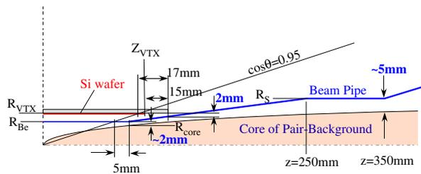
Figure 2: Model for estimation of radii of the beam pipe and innermost layer of the GLD vertex detector.
