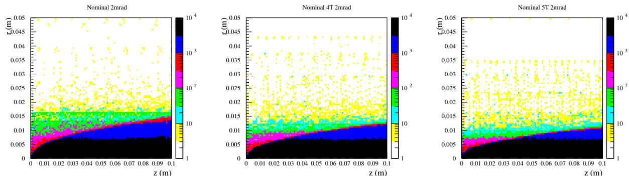
Figure 3: Pair-background track density ( $1/\text{cm}^2/\text{BX}$ ) with the nominal ILC machine parameter at 500 GeV and 2 mrad crossing angle in 3 T (left), 4 T (center), and 5 T (right) magnetic field.
