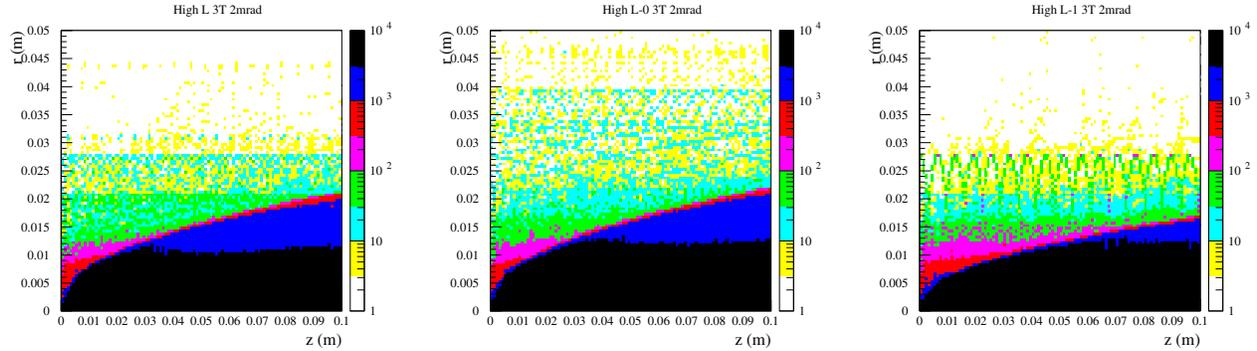
Figure 4: Pair-background track density ( $/\text{cm}^2/\text{BX}$ ) with the high luminosity option of ILC machine parameter at 500 GeV (left), 1 TeV (center) [1], and the new high luminosity option at 1 TeV [2] (right). The crossing angle is 2 mrad and the magnetic field is 3 T for all three cases.
