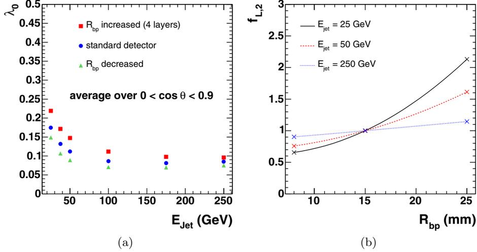
Figure 2: Comparison of detectors with different beam pipe radius: (a) in terms of their leakage rates and (b) in terms of the 2-jet luminosity factor compared to the standard design, see text.
