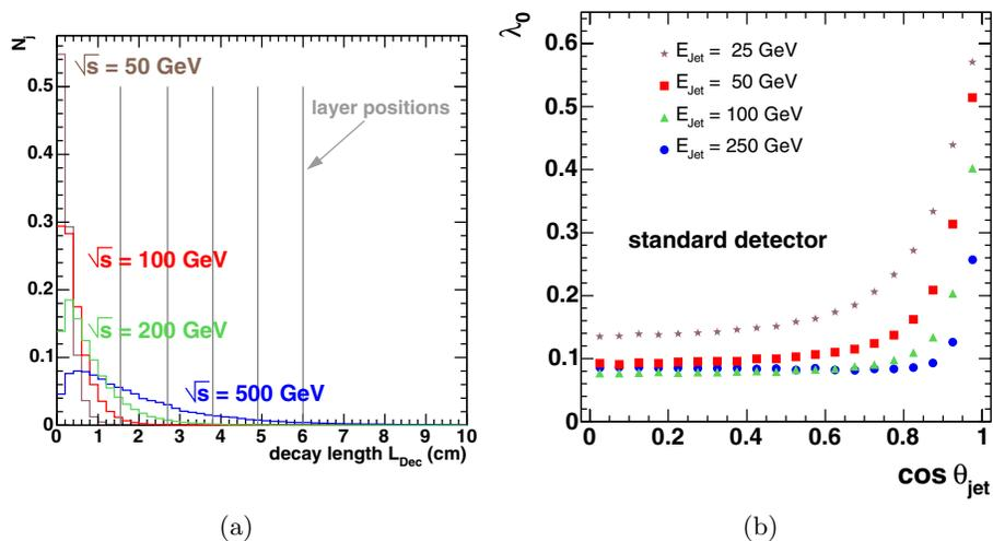
Figure 1: (a) Decay length distribution for outermost reconstructed vertex in jets from  $e^+e^- \rightarrow b\bar{b}$  events. (b) Probability  $\lambda_0$  of misreconstructing neutral vertices as function of jet energy and polar angle.
