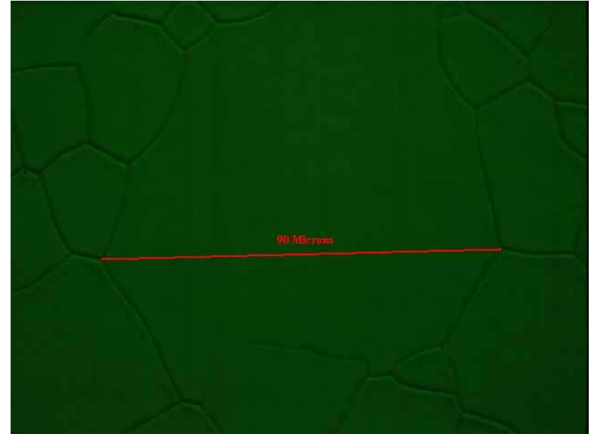
1000 x showing 90 \mu\text{m} crystal (previous maximum = 15 \mu\text{m} )
