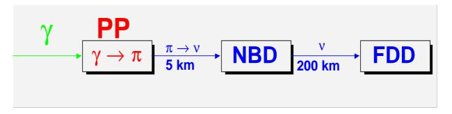
A. Pion producer (PP) – water cylinder of length about 20 cm (radiation length). Here electrons produce photons via bremsstrahlung, and than these photons (or direct photons) produce pions via  $\gamma N \to \pi\pi\pi...N$
