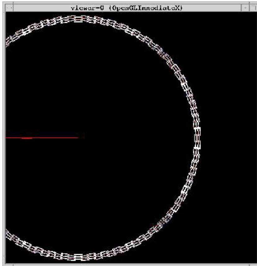
Silicon Tracker Envelope in Mokka (G4) framework (V. Saveliev)
