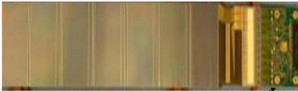
28 cm long Si strips prototype tested with VA front-end
