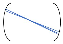
Light in narrow focusing cavities tends to a particular point on the mirror
