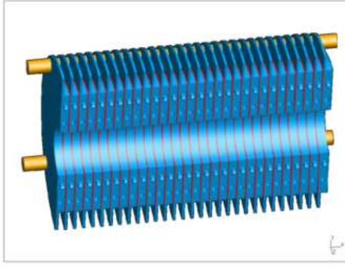
Figure 1: The structure of a half barrel of the sandwich calorimeter. Between the tungsten disks diamond sensors are interspersed.
