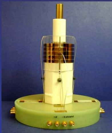
Inner electrode structure surrounding test mass. Electronic hardware interface measurements underway since April 2001
