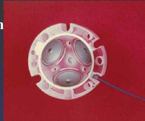
GP-B Pickup Loop: 4 turn Nb Electrodes and Ground Plane
