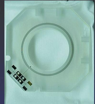
STEP Pickup Loop: 5 turn Nb plus Integrated Heat Switch
