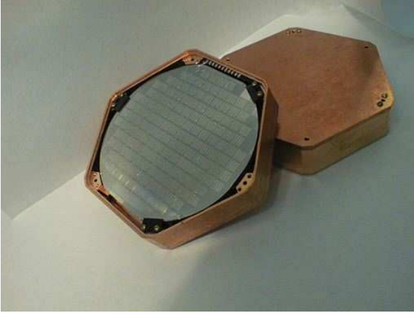
Figure 1: A CDMS II ZIP (Z-sensitive Ionization and Phonon) detector and its housing. Data for this analysis were taken with a single “tower” of six such detectors.
