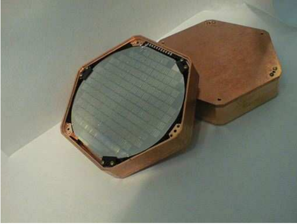
Figure 1: A CDMS II ZIP (Z-sensitive Ionization and Phonon) detector and its housing. Data for this analysis were taken with a single “tower” of six such detectors.
