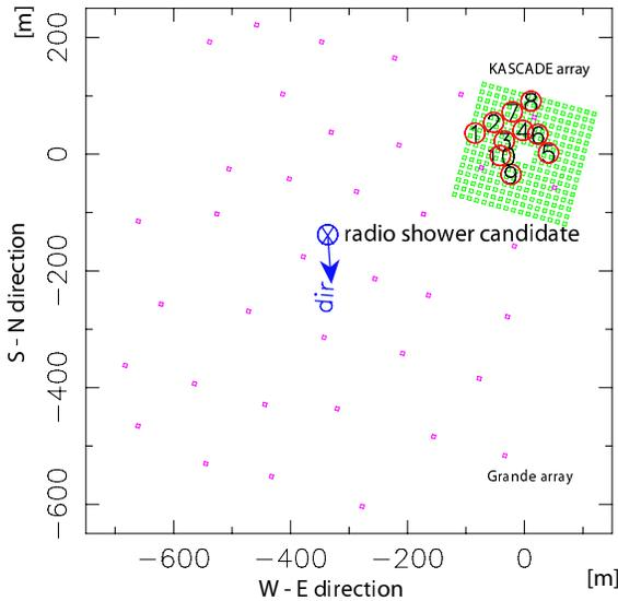
Figure 6: Layout of LOPES 10 in respect to the KASCADE-Grande experiment. The marker denotes core position and direction of a promising radio event.
