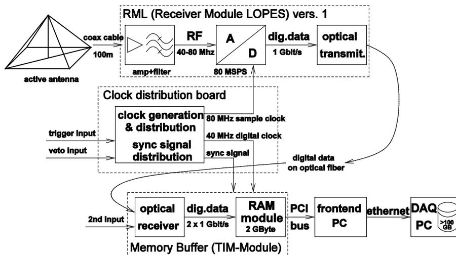
Figure 3: Layout of the LOPES hardware components.
