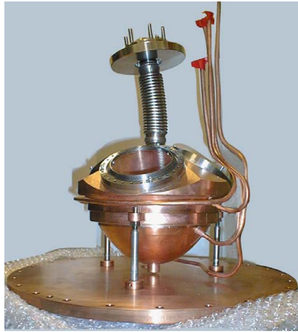
Figure 11: Photograph of the ZEPLINI inner liquid xenon detector.
