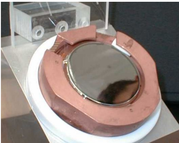
Figure 7: Photograph of a 320 g EDELWEISS germanium bolometer.
