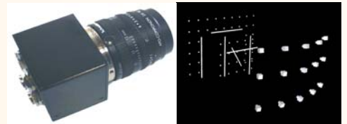
SVS4020 industrial 4-Mpixel camera (source: SVS-Vistek GmbH) Test field and camera positions
