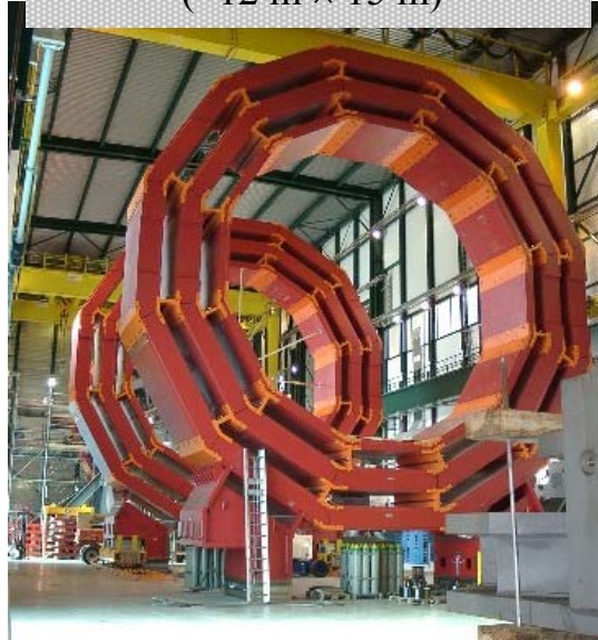
Wheel: three concentric iron layers.
