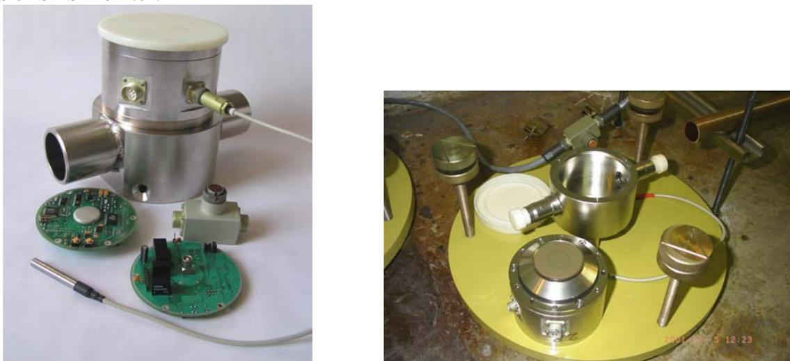
Fig.12 Partly disassembled SAS monitors
