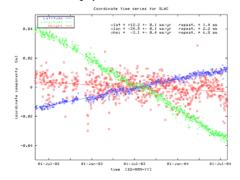
The daily solutions of the regional network were transformed onto the ITRF2000 reference frame by means of a six-parameter Helmert transformation (no significant scale parameter). The velocities of the 3 coordinate components latitude, longitude, and height are estimated by fitting a linear trend to the data.
