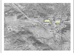
24-hour sessions have been observed on the SLC stations using Leica SR530 receivers and Leica AT-503 antennas. The 4 Linac penetration points (M1, M10, M19, and M42) were set up on translation stages with the AT-503 centered over the ground point by means of a nadir plummet. For these stations no height reference was established.
