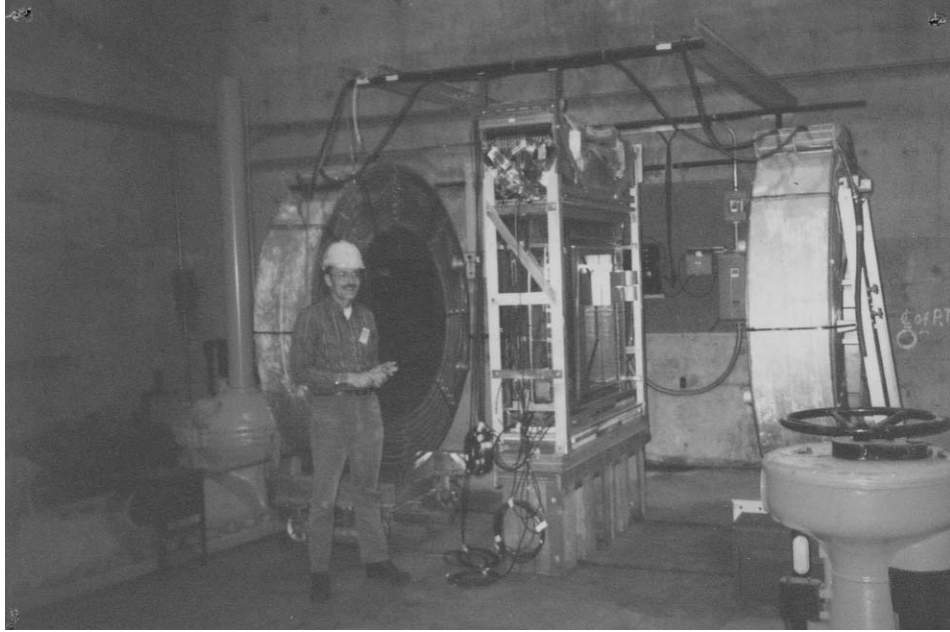
Figure 3: Michael Moe is shown standing by the time projection chamber used for the first direct observation of \beta\beta(2\nu) [1].
