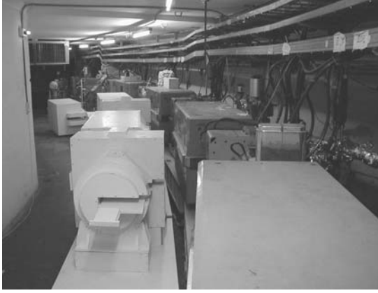
Figure 6: Mock-up of two rings in the BEPC tunnel
