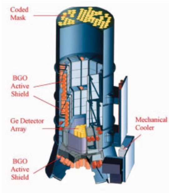
Figure 2: INTEGRAL Spectrometer (SPI)
