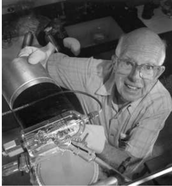
Figure 1: Ray Davis preparing to pour liquid nitrogen into a dewar on a vacuum system of the type used for gas purification and counter filling in the chlorine experiment. The glass object in the foreground with the wire coming out that blocks Ray's left hand is an ionization gauge used to measure the pressure in the vacuum system.
