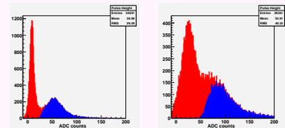
Pulse distribution from Si strip detectors. The right plot shows the pulse distribution of the studied Czochralski detector. Red color displays data after level 1 selection and the blue color displays data after level 3 selection.
