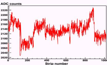
Pedestal spectrum of a silicon strip detector. The differences of the 8 VA1 chips are clearly visible.
