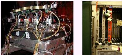
Silicon Beam Telescope (left) and Commercial VME modules of DAQ: VME-PCI interface, ADC and scaler unit (right)
