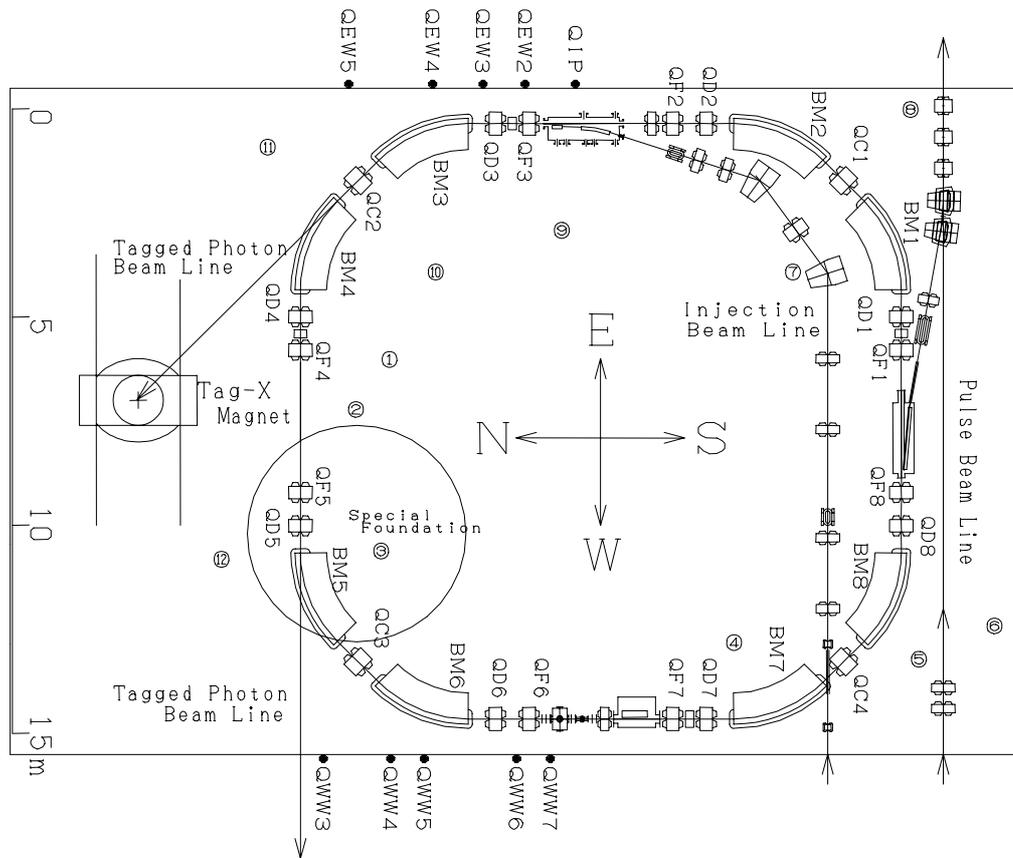
Fig2 The STB ring in the experimental hall No.2. A circular mark on the BM5 shows a part of the base which was separated from the floor of the hall. Small circular marks with numbers show setting points of surveying poles. QIP, QEW and QWW on the east and the west walls are marking points on the walls.
