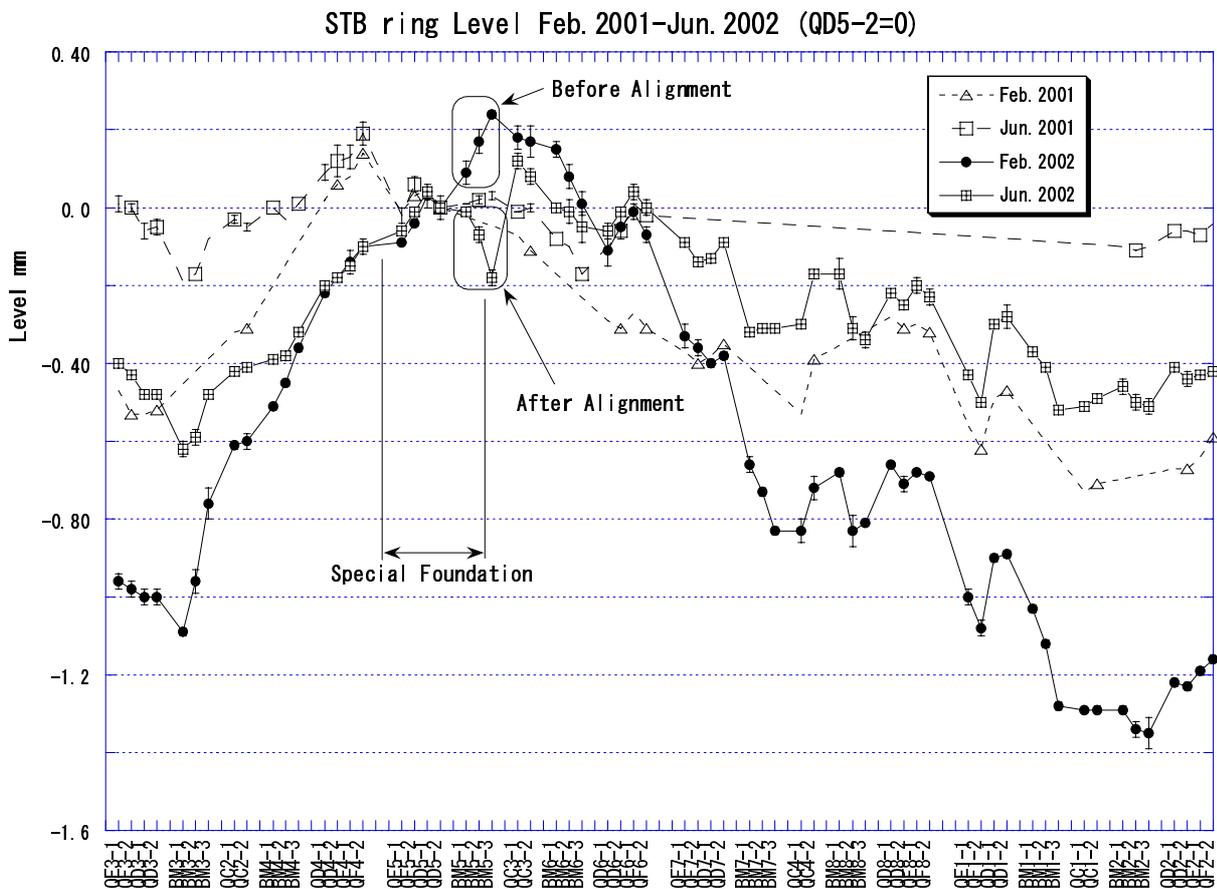
Fig.7 Level data from February, 2001 till June, 2002 plotted relative to QD5-2. The Data of 2002 are shown by solid line. The circular marks in the figure denote before and after the BM5 re-alignment.
