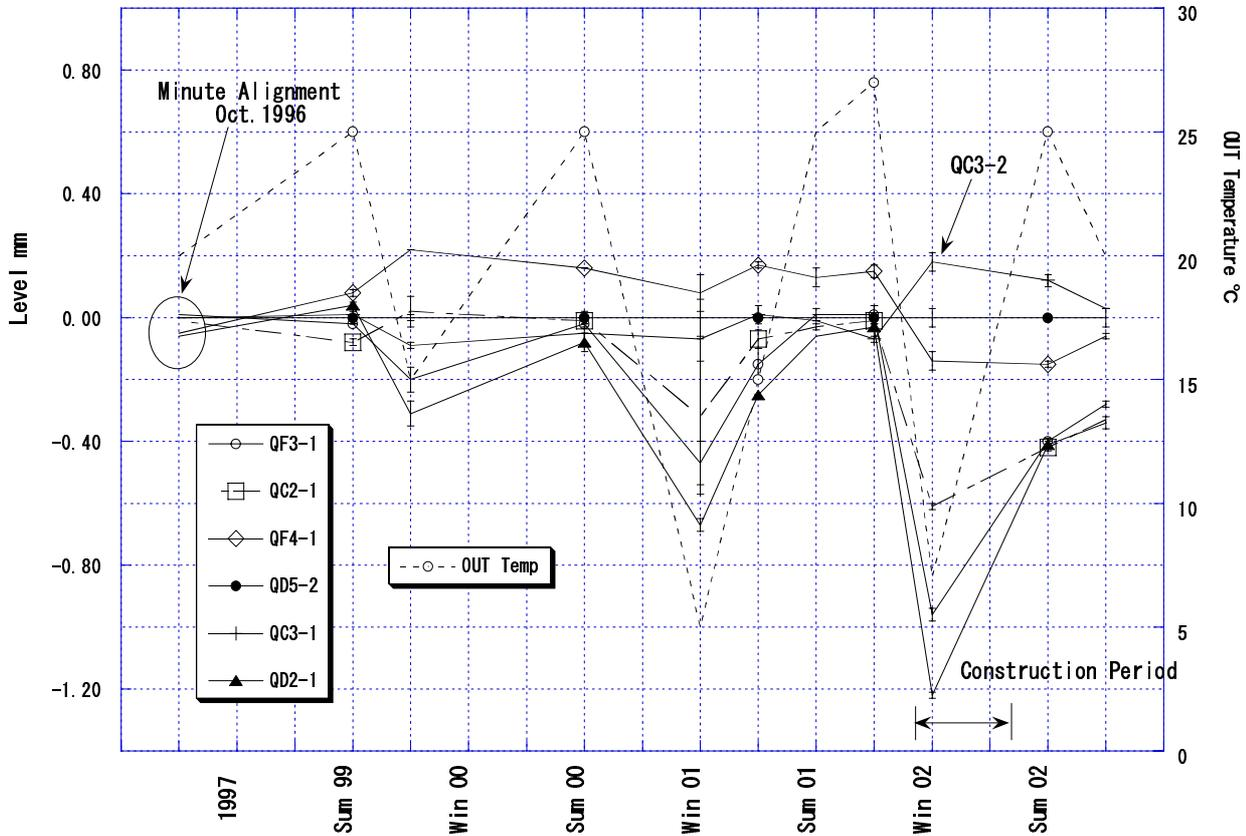
Fig.8 Periodic seasonal variations of the magnets level in the ring until now. QC3-2 (in the side of the west wall) is raised, and other magnets go down greatly in February, 2002 term because of the influence of the new experimental hall construction.
