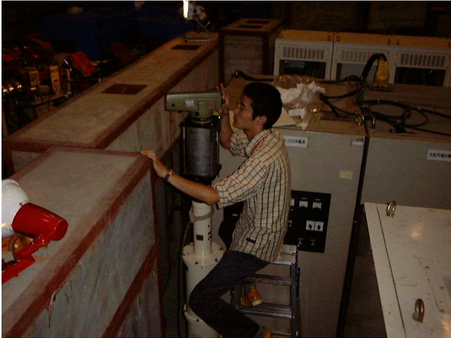
Fig.4. The scenery of the surveying at the east side straight section of the ring. The height of the standard target for the aiming is set to be 2.2 m because of the 2.0 m-tall radiation shields inside of the ring.
