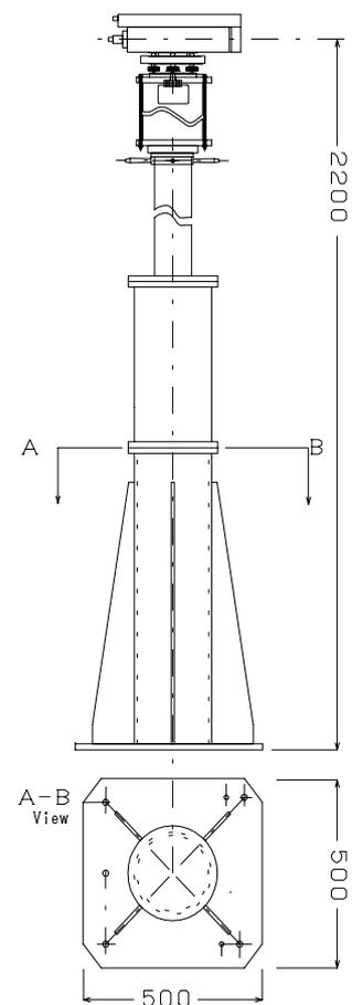
Fig.3 A pole for level survey. It is made of iron-steel of about 100 kg, the height of 2.2 m can take aim at the targets.
