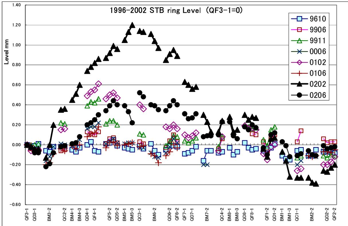
Fig.5 Measured magnet level plotted by setting the level of QF3-1 to be zero. An indication 0202, for example, means measured in February, 2002.
