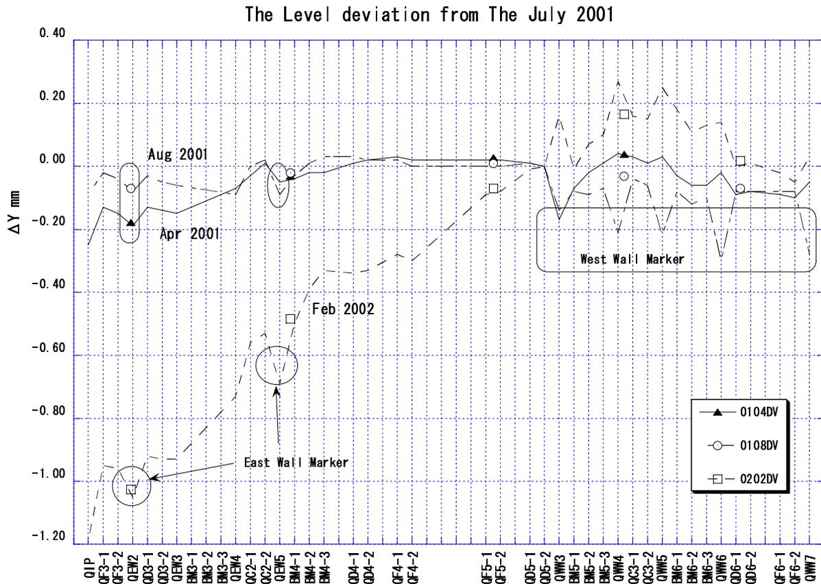
Fig.6 The deviation of each surveying term relative to the data on June, 2001 is shown for the north straight section.
