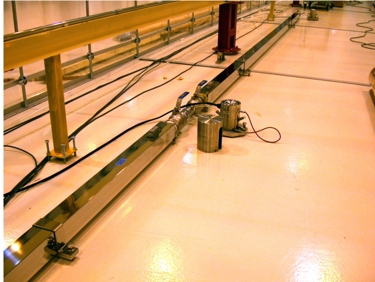
Fig.11 Ten meters of movable HLS were set in the experiment hall for testing.
