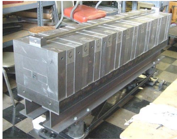
Figure 11. The complete collimator including the clamping bar.
