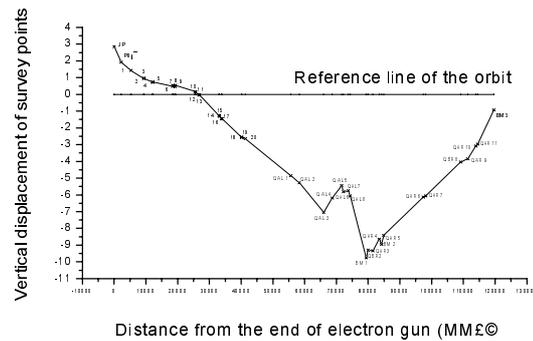
Fig.5 Absolute vertical displacement of the points
