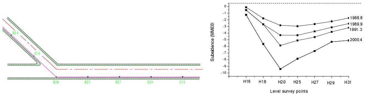
(a) Level survey points along the tunnel
