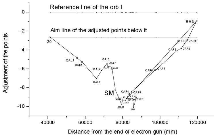
Fig.6 Adjusted points and the displacement
