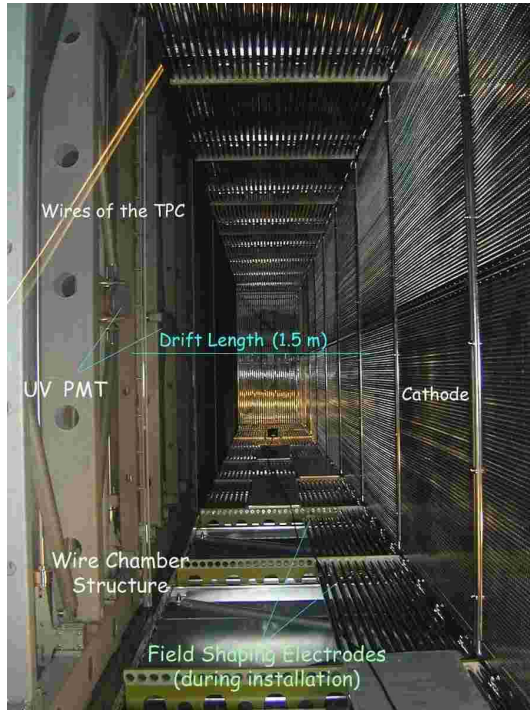
Figure 6. Internal view of the T600 first half module.
