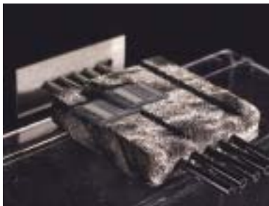
Figure 2: Prototype fuzzy carbon substrate with embedded cooling lines.
