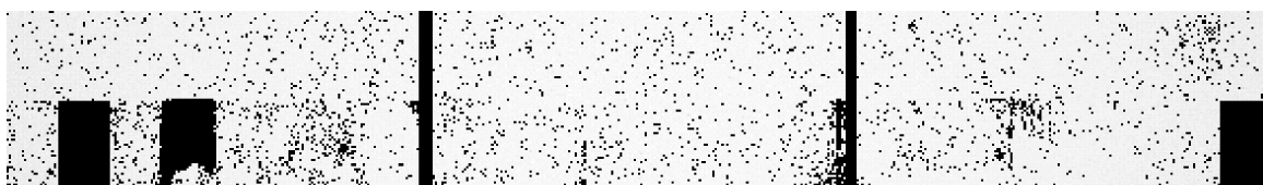
Figure 3: Flat-field corrected image of Br fluorescence x-rays (11.9 keV) recorded with the single bank detector. The 11 pixel gaps between the modules are seen as black columns. Black pixels are defective. Three chips have partial or total electrical or bump-bonding failure. The flat field correction takes into account air absorption, angle-of-incidence correction, and silicon absorption. Each pixel received 1.2 \times 10^4 x-rays in this 40 s exposure. The left and right edges of the image are slightly darkened because of the 1/r^2 falloff of the illuminating field.
