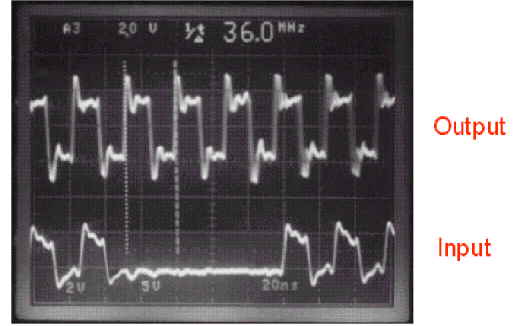
Figure 9: Scope trace of the input and output of the PLL chip demonstrating clock recovery.
