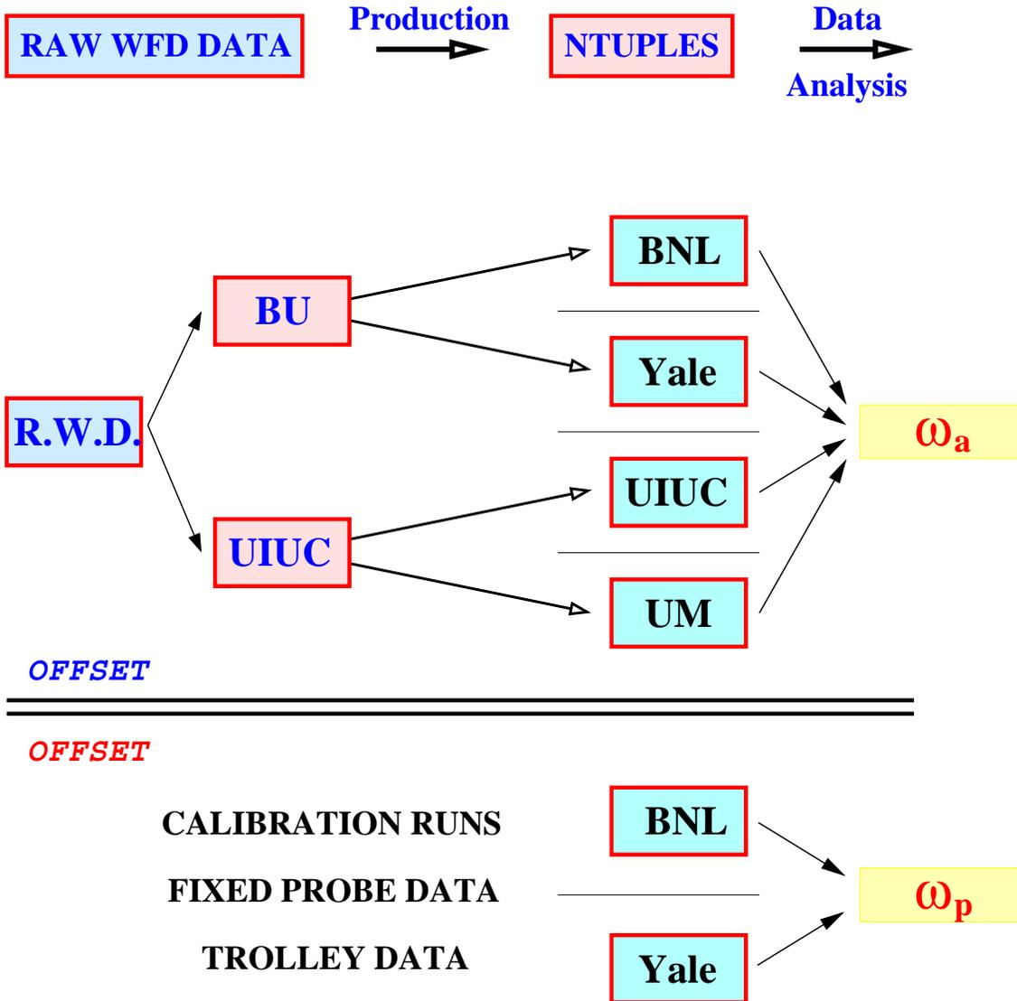
$$a_\mu = \frac{\frac{\omega_a}{\omega_p}}{\lambda - \frac{\omega_a}{\omega_p}} \quad \lambda = \frac{\mu_\mu}{\mu_p} = 3.183\ 345\ 39(10)^*$$
