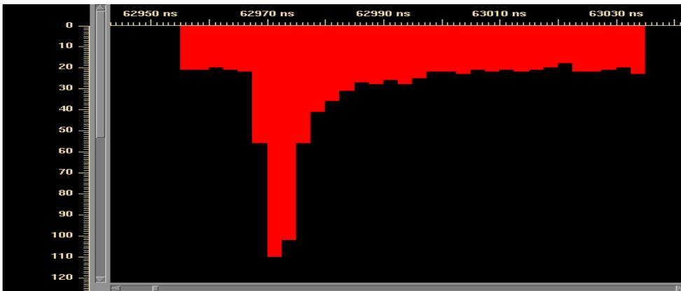
If there are pulses after the main triggering pulse on the same island (shadow pulses).
