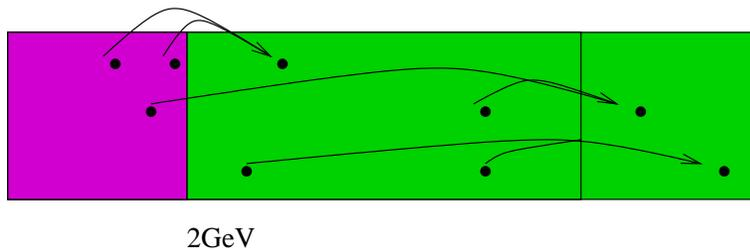
An early to late effect caused by the change on muon intensity (due to decay) and enhanced by the Fast Rotation Factor
