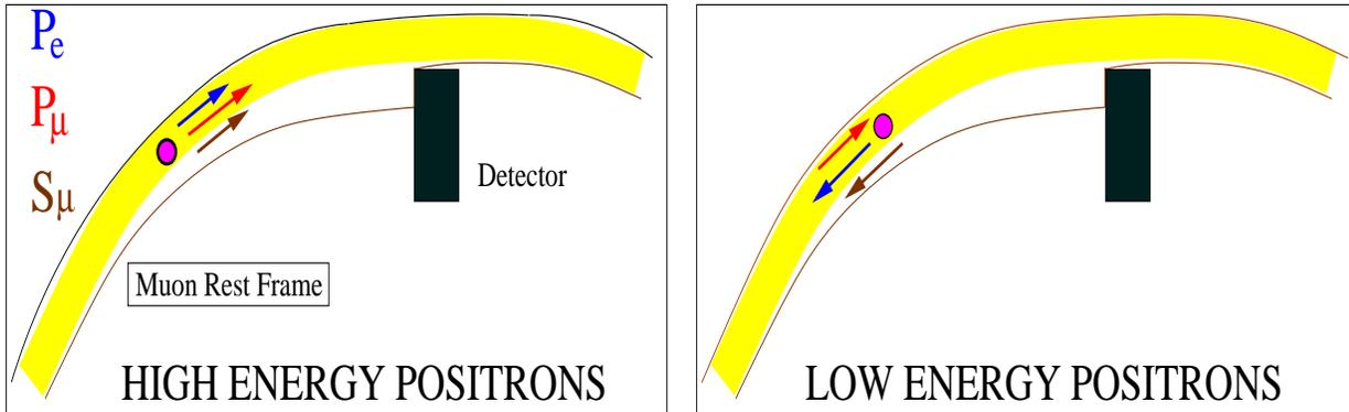
$S_\mu$  is precessing in the field  $\rightarrow e^+$  counting rate is modulated with the  $\mu$  spin precession
