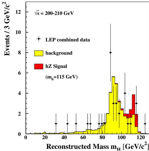
Figure 2: Distribution of the reconstructed Higgs boson mass,  $m_H^{\text{rec}}$ , obtained with a special, non-biasing, selection. The cuts are adjusted in such a way as to obtain approximately equal numbers of expected signal and expected background events in the region  $m_H^{\text{rec}} > 109$  GeV.
