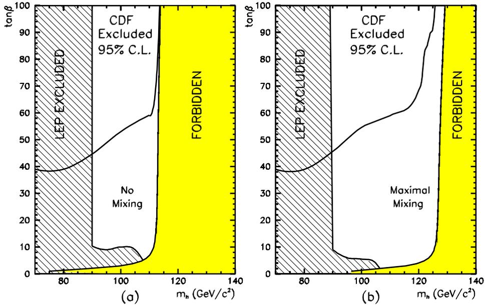
Figure 10: The 95% C.L. excluded regions in the  $(\tan\beta, m_h)$  plane for the two scalar top mixing scenarios : a) “no mixing”, b) “maximal mixing”. Results are obtained by the CDF collaboration. The LEP excluded regions shown here are obsolete.
