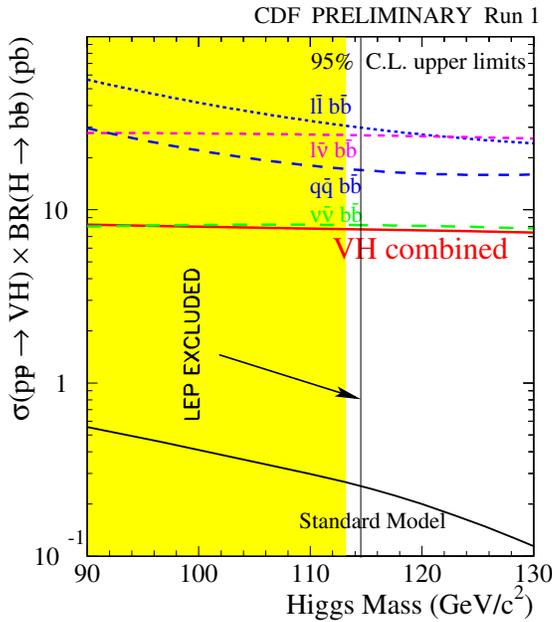
Figure 4: The 95% C.L. upper limit set by CDF on the product of the HV (V is W and Z) production cross section and the branching fraction of  $H \rightarrow b\bar{b}$  compared to the SM prediction. Also shown is the combined LEP limit.
