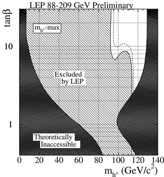
Figure 9: The 95 % C.L. exclusion contours in the  $(\tan\beta, m_h)$  projection for the “ $m_h - \max$ ” scenario. The results of the four LEP experiments are combined. The hatched area is excluded, the filled area is theoretically inaccessible and the dashed line indicates the expected boundary of the excluded region in the absence of a signal.
