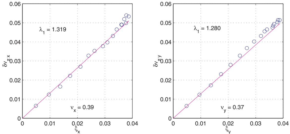
Figure 2: (color) The tune shift of coherent  $\pi$  mode as a function of the beam-beam parameter. The left plot is for the horizontal plane and right plot is for the vertical plane. The circles represent the simulated tune shifts. The solid lines represent  $\delta\nu_\pi = \lambda\xi$  derived from the Vlasov theory.
