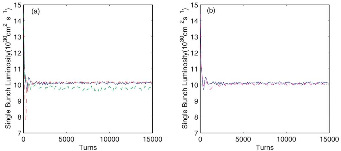
Figure 3: (color) (a) The dashed green curve is the case when  $N_b = 10^4$ , the solid blue curve is for  $10^5$ , and the dash-dotted red curve is for  $10^6$ . (b) The solid blue curve is for the mesh  $64 \times 128$  and the dash-dotted magenta curve is for the mesh  $128 \times 128$ .
