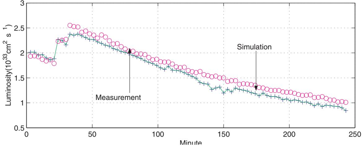
Figure 1: (color) Luminosity of PEP-II. The crosses represent measurement and the circles represent simulation. The number of bunches was 605.
