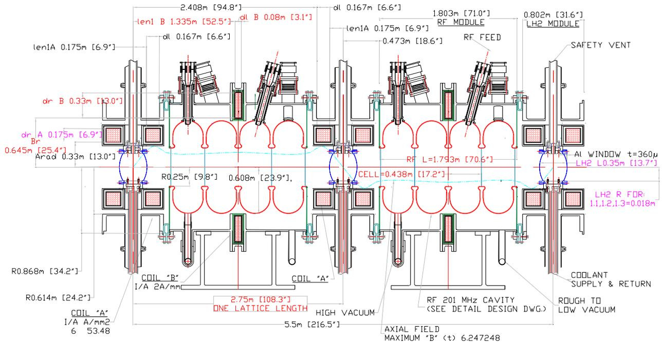
Figure 1: SFOFO ionization-cooling lattice (from [15]).
