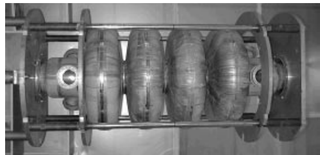
Figure 5: The prototype 4-cell \beta=0.7 cavity
