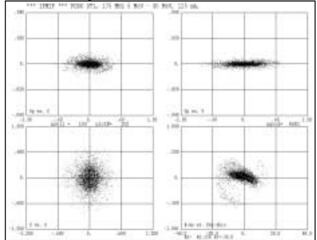
Figure 2: Output emittance of the 175 MHz DTL with direct input from the RFQ 3 from Table 2 and a 6.2 cm drift between RFQ and DTL.
